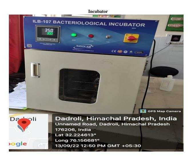
**Principle** - Themain principle of incubator is to maintain condition of temperature and humidity inside the chamber in such way that it forms favourable condition for rapid multiplication of microbial cells. It can be adjusted in such a way that only desired cells are able to replicate and rest of others fails to survive and hence get vanish.
