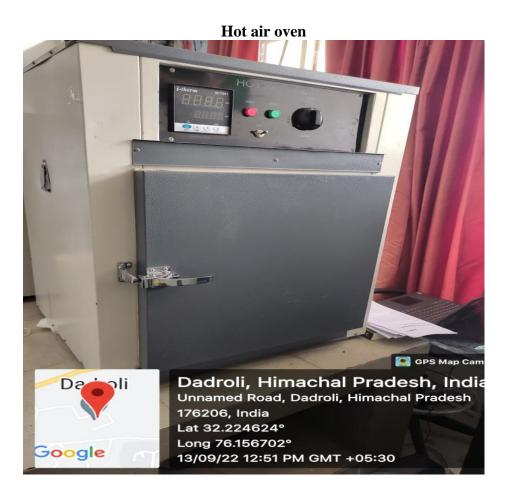
**Principle**: It is based on sterilization by dry heat is performed by conduction. The temperature is consumed by the surface of the objects, then moves towards the core of the object, coating by coating. The whole object will ultimately attain the temperature needed for sterilization to take place
